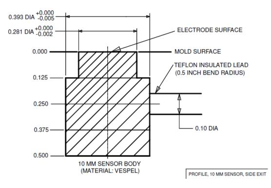
Figure 4 Nominal dimensions of 10-mm Unitrode, side exit
