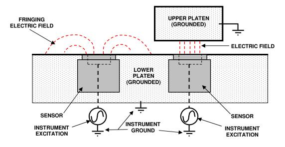
Figure 3 10 mm Unitrode sensor using nearby grounded surface as second electrode
