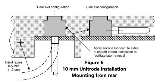
It is important to support the bottom plate of the sensor to prevent high pressures from pushing it out of position. To facilitate removal when necessary, silicone lubricant may be applied to the side of the sheath before installation.
