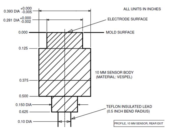
Figure 5 Nominal dimensions of 10-mm Unitrode, rear exit
