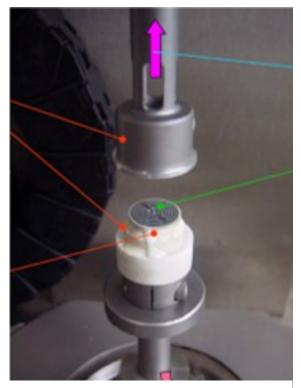
Figure 7-1 Simultaneous DMA-DEA apparatus
