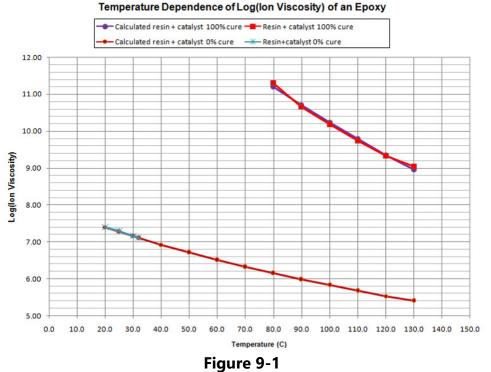
Variation in log(*IV*) with temperature for an epoxy resin
