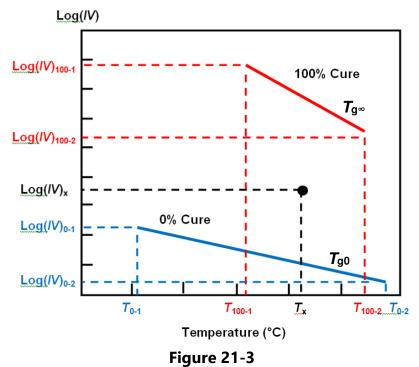
Cure Index baselines with ion viscosity-temperature data point
