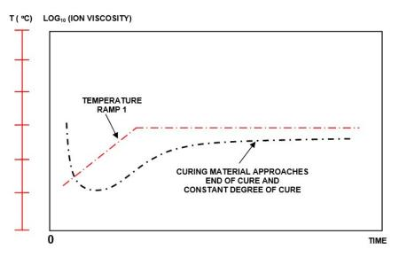
Figure 21-6 Ion viscosity during cure
