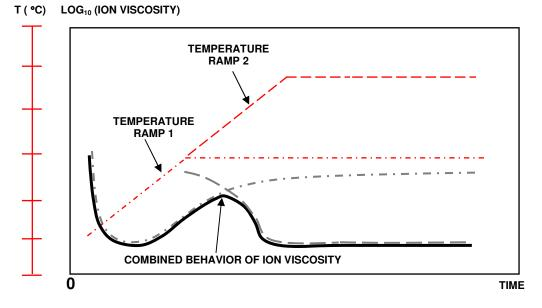
Figure 21-10 Ion viscosity response to a single ramp and hold step
