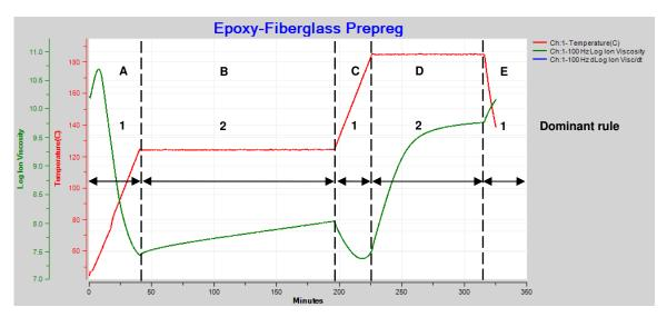
Figure 21-1 Epoxy-fiberglass prepreg cure with ramps and holds
