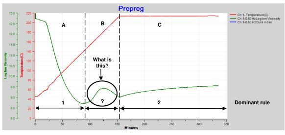
Figure 21-2 Epoxy-fiberglass prepreg cure with ramp and hold
