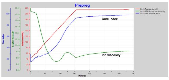
Figure 21-5 Epoxy-fiberglass prepreg ion viscosity and Cure Index
