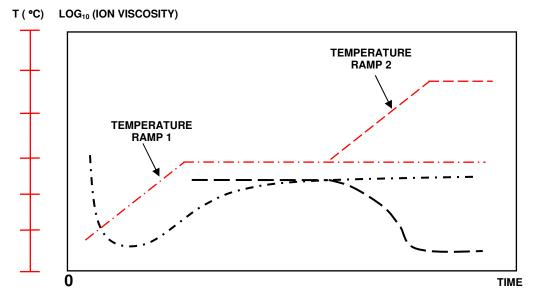
Figure 21-8 Ion viscosity response to two ramp and hold stages
