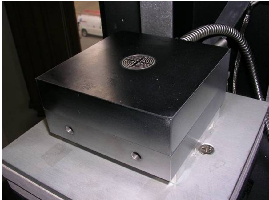
Figure 39-6 Ceramiccomb-1'' sensor in press platen, A/D = 10 cm
