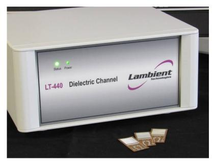
The LT-440 Dielectric Channel, an upgrade of the LT-439, is a cost effective, compact instrument designed for cure monitoring in R&D, Quality Control/Quality Assurance and manufacture of thermoset materials—resins, composites, paints and coatings. The LT-440 will accept all Lambient Technologies dielectric/conductivity
