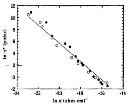
Figure 1-4 Viscosity vs. conductivity (ion viscosity = 1/conductivity) for an epoxy<sup>2</sup>
