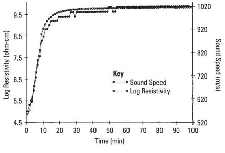
Figure 1-6 Resistivity (ion viscosity) vs. sound speed for a curing epoxy-fiberglass prepreg<sup>4</sup>
