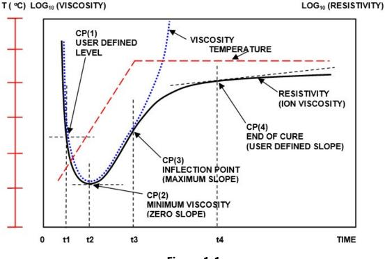
Figure 1-1 Ion viscosity and mechanical viscosity for thermoset cure
