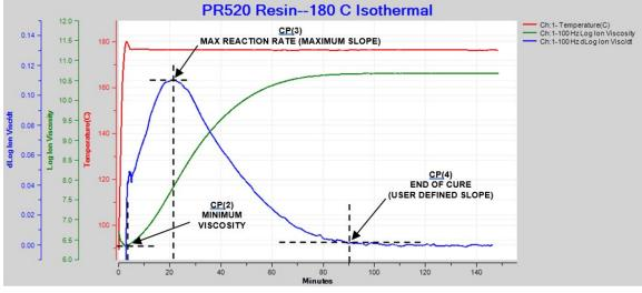
Figure 1-3 Ion viscosity and slope of ion viscosity for thermoset cure during isothermal processing
