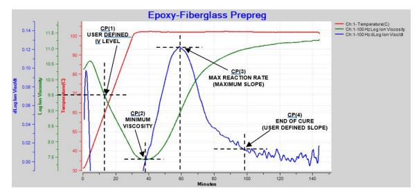
Figure 1-2 Ion viscosity and slope of ion viscosity for thermoset cure during thermal ramp and hold
